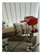
The facility can be operated at a defined vacuum pressure, ranging from the 10<sup>-5</sup>mbar range to ambient pressure, under defined gas atmosphere (air, inert gas, specific gas atmosphere such as Martian atmosphere). Corrosive atmosphere is currently not feasible.
